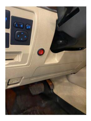
The red button in the above picture is an emergency button. It is located below the steering wheel to the left of the driver. This button sends a signal to the carpooling administrator to alert him in case of emergency. Please keep it "off" when there is no need to use it.
