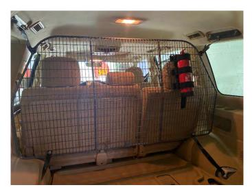
The main purpose of the protection net is to prevent the movement of items from the trunk to the passenger compartment. Fire extinguisher and first aid kit are mounted on the net in a way that does not prevent the visibility of the rearview.
