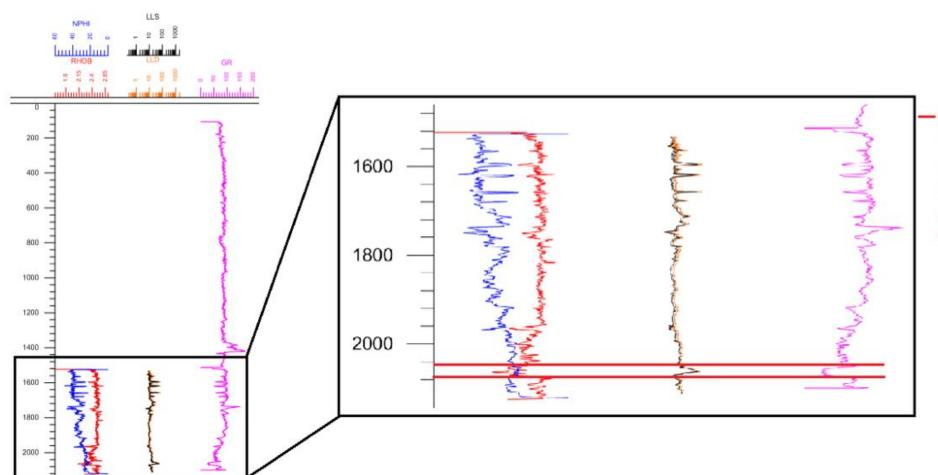
A sandstone reservoir, indicated by low gamma ray, RHOB-NPHI cross over, and high resistivity value. This is an oil reservoir (NPHI not too low).
